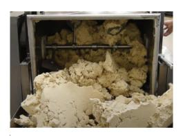
Turn on the equipment so that the dough comes out of the hopper
