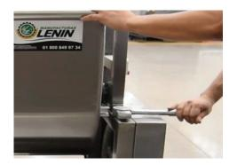
7 Turn lever to release the hopper
